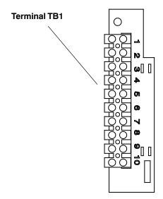
Figure 5-3. EMB(0) Control Connector
