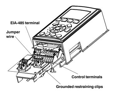
Figure 3-10. Control Terminals Location
