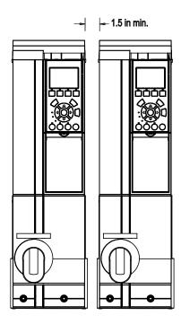
Figure 3-4. Side Cooling Clearance, A-2 and A-3 Frames
