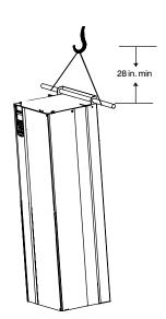
Figure 3-3. Proper Lifting Method
