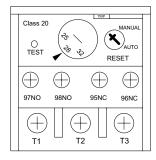
Figure 5-5. Sample Overload Device
