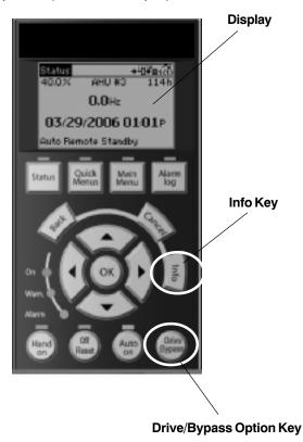
When running in drive mode, press OK key on keypad to activate bypass mode or press CANCEL to remain in drive mode. In bypass, motor will run at full speed.
