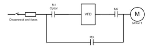
Figure 1-1. Basic 3-contactor Bypass Functions
