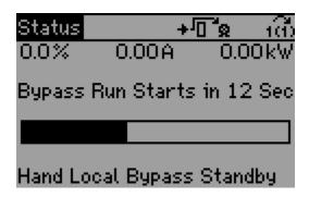
Drive Display with Bypass Start Time Delay Active
