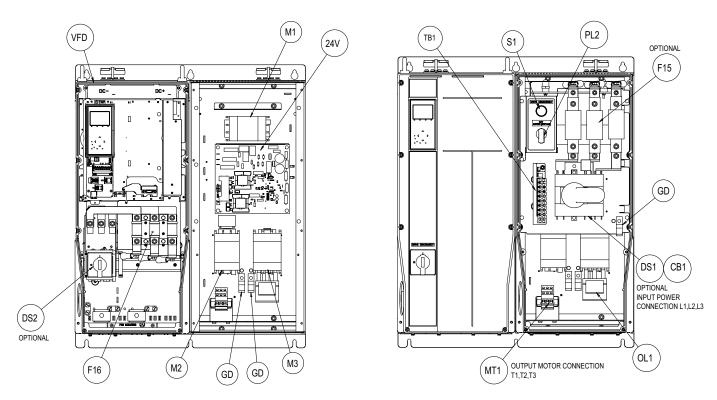
Figure 3-7. Sample Mechanical Layout Diagram
