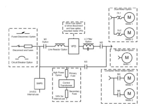
Figure 1-2. Bypass Curcuit with Options
