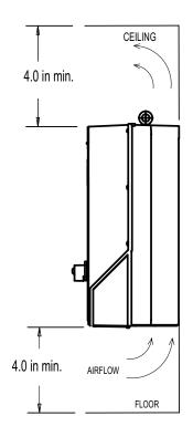
Figure 3-5. Cooling Airflow
