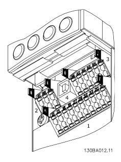
Figure 6-2. Drive Control Terminals
