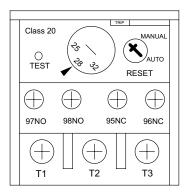
Figure 6-4. Sample Overload Device
