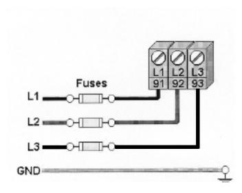
Figure 3-1. Drive Input Fuses
