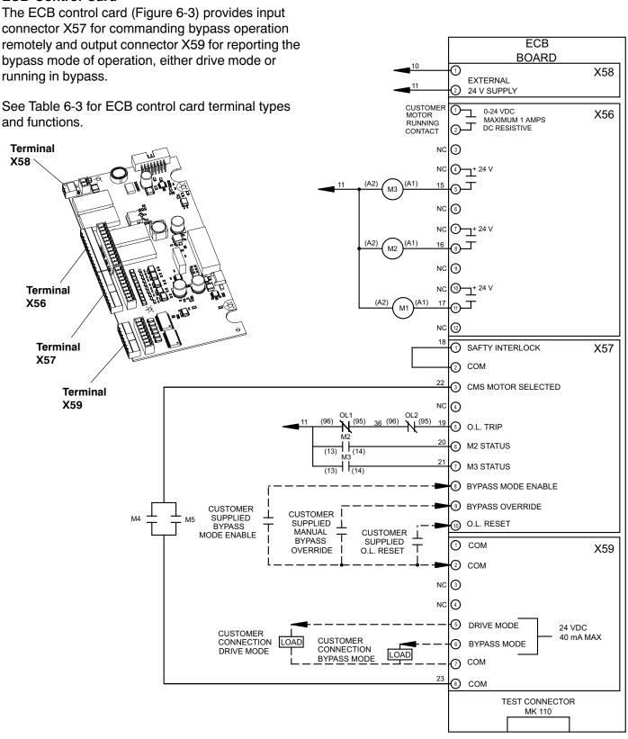
Figure 6-3. ECB Control Card Terminal Connections
