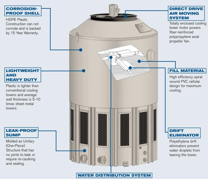
Self-propelled multiple PVC rotating arm system evenly distributes the water.
