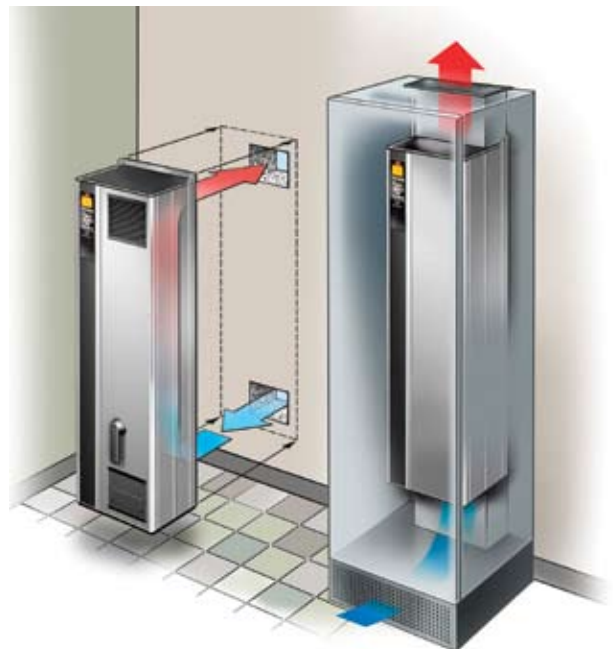
Back-channel cooling: A smart, dedicated kit allows chassis/IP00 enclosures to be mounted in Rittal cabinets so cool air removes 85% of excess heat without contact with the electronics.
