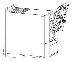
Step 3 Push the top of the LCP into the drive
