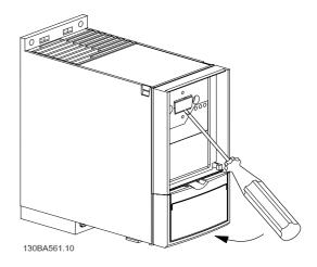
Step 2 Place the bottom of the LCP in the drive
