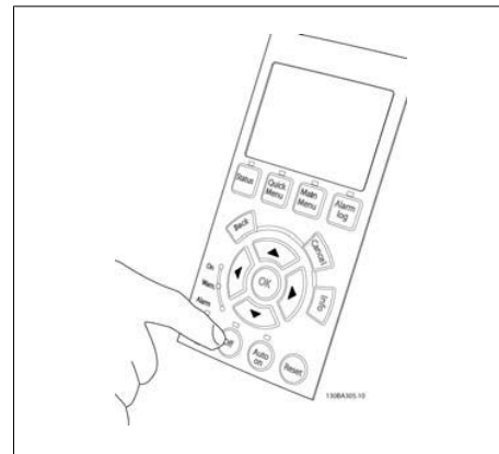
5.22: Step 4: Power up the unit and press the [Off] button. In this state, the motor should not rotate. Press [Off] to stop the motor at any time. Note that the LED on the [OFF] button should be lit. If alarms or warnings are flashing, please see chapter 7 for more information.
