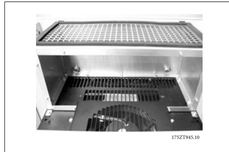
3.42: Top duct installed
