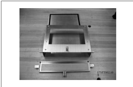
3.52: Bottom duct work partially assembled
