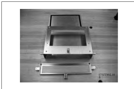
3.52: Bottom duct work partially assembled
