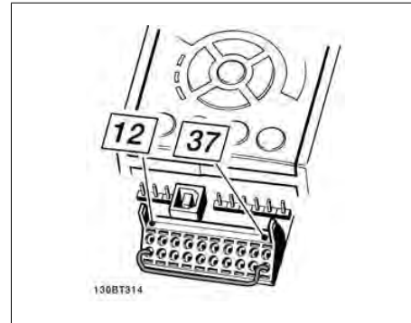
2.1: Bridge jumper between terminal 37 and 24 VDC
